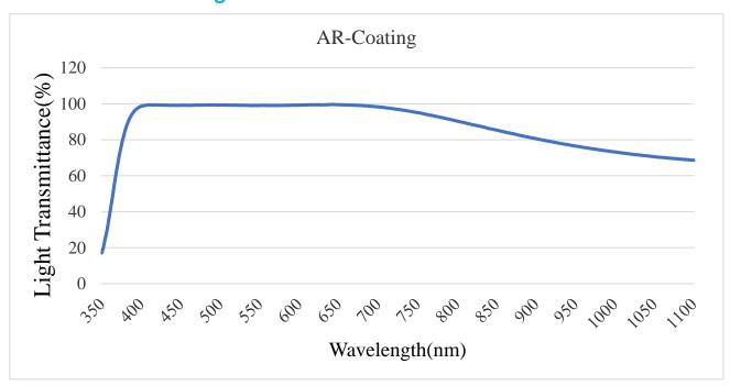
The window is coated with an anti-reflective layer, providing over 99% light transmittance across the 400nm to 680nm wavelength range, effectively minimizing interference from secondary reflections and enhancing system stability.
