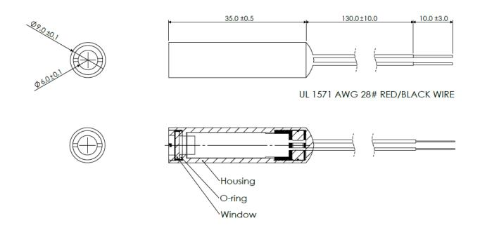
The laser module is installed within a housing through a specially designed mechanism, with the front end sealed by O-ring and window, and back end sealed with epoxy, ensuring waterproof capabilities.
