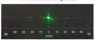
LM4 series beam shape at 3m
