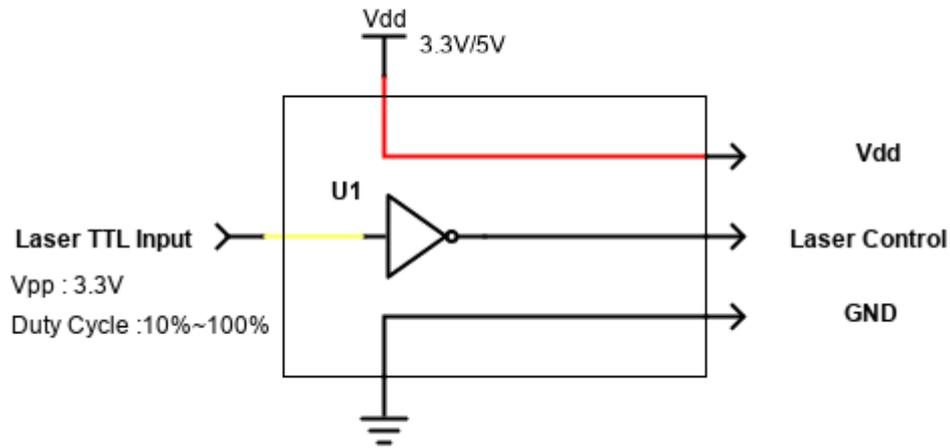
All TTL control laser modules will be prepared with 3 flying leads. In addition to red wire for power & black wire for ground, yellow wire allow users to provide programmed PWM signals to tune laser power output. Recommended duty ratio ranges from 10% to 100%.
